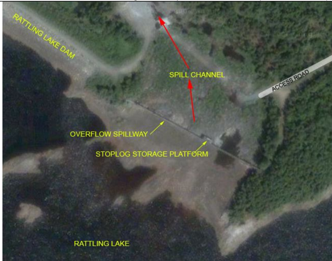
Figure 3 - Existing Site Layout
